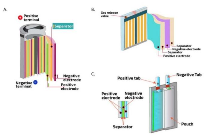
Schematics of various form factors for Li-ion cells, including: A) cylindrical, B) prismatic, and C) pouch. *Source: Sandia National Laboratory*. <u>Click to enlarge</u>.
